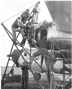
Fig. 40 The powerful engines were replaced after the required number of running hours.
