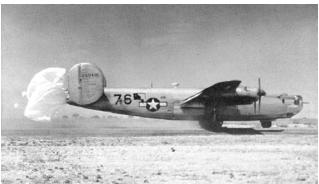
Fig. 38 Left: Damaged hydraulic systems caused parachutes to be used to help slow this plane upon landing. The parachutes were attached to the waist machine gun mounts, and opened after the plane landed.
