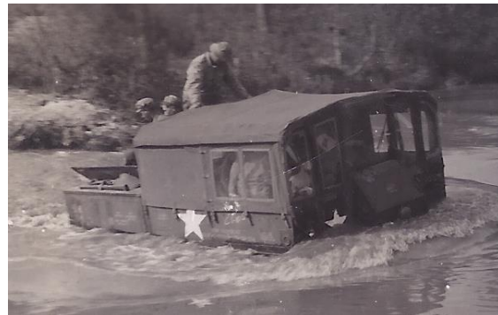
Testing Air breathing "Snorkel" for deep water beach landing.
