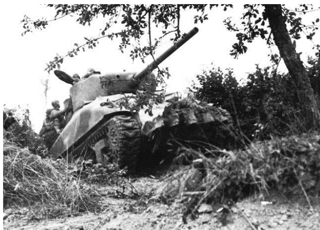
Tank modified with iron teeth, cuts through the bocage.
